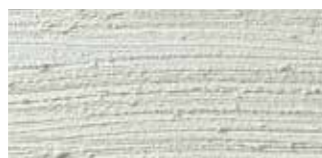
Broom coating technique
